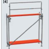
The Permanent Advanced Guardrail guardrail for **SUPER** and **FRAMESCAFF** is placed on the top tube connector of a vertical frame from the lower scaffold level [1], the handle is released [2], the guardrail folded out [3] and latched in [4].
